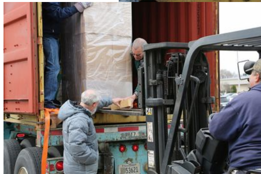
◀ Each transmitter was tilted, then blocked, to allow the forklift to get under the transmitter.
