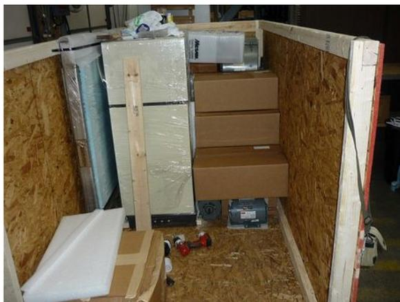
Heavier items (like the radiator and regulator on the left and motors and transformers on the bottom) were secured in place first, then boxes packed around them.
