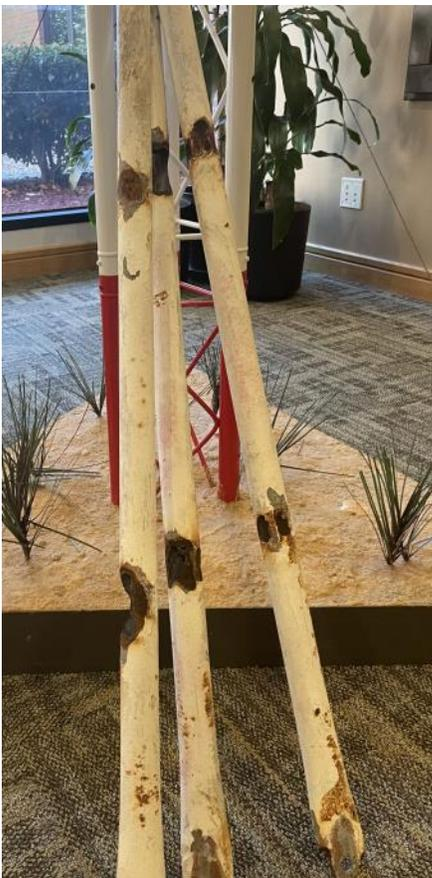
These are tower cross braces from KTWR. As you can see, they are rusted through and have been replaced. There are 2500 more that need replaced.
